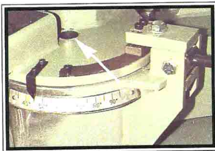
Swivel Pivot pin fitting under dome cap.
