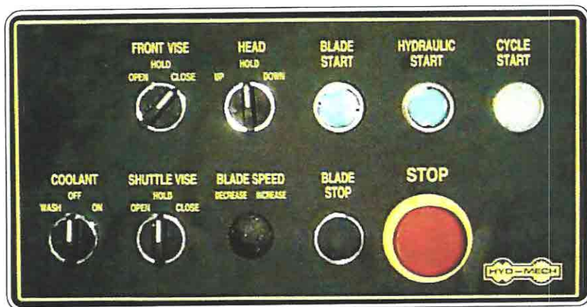
Manual Control Switches for PLC 100
