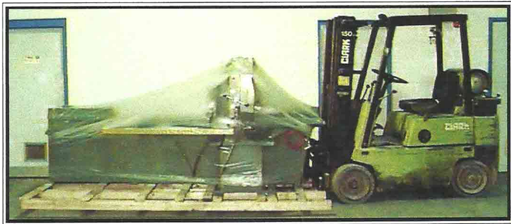
Lifting the S-20A Series II with a Forklift Truck
